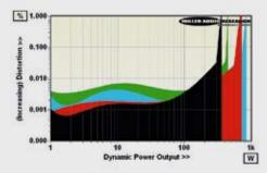
ABOVE: Dynamic power output versus distortion into 80hm (black trace), 40hm (red), 20hm (blue) and 10hm (green) speaker loads. Max. current is 22.3A
