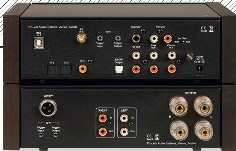
ABOVE: Line and phono analogue ins are offered alongside coax, USB, wireless Bluetooth and two Toslink optical digital ins, with fixed/variable analogue, sub plus optical outs [Pre Box, top]. The Amp Box [below] has line in/loop outs on RCA and 4mm speaker terminals. Note the three-pin DIN 48V PSU connection
