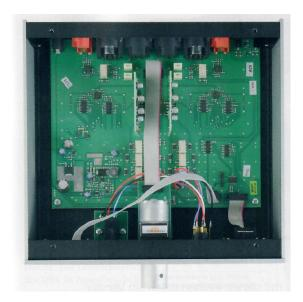
Left: The double mono structure of the amplifier circuit can be clearly seen. The omission of further features explains the airy equipped board of the Head Box DS2B.
