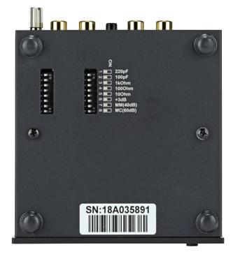
Two rows of recessed DIP switches – one per channel – enable Phono Box S2 Ultra to be 'matched' to whatever cartridge (MM or MC) you happen to be using. A tiny screwdriver is needed to flip each switch.
