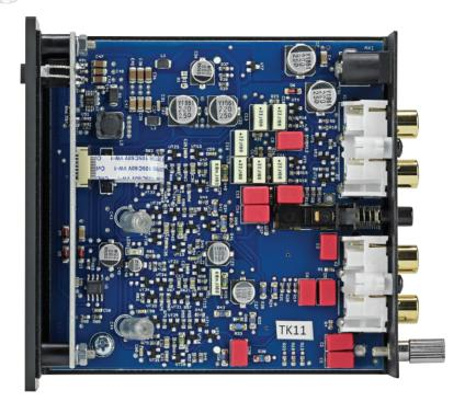
The circuit board of the Phono Box S2 Ultra is busy, full of transistors instead of generic op-amps. Decent-quality passive components, like polystyrene capacitors, are also in evidence. According to Pro-Ject "the split RIAA equalization" implemented with this collection of devices "enables a pin-point accurate representation of the RIAA curve" to be achieved. The unit's only chips are power supply components.
